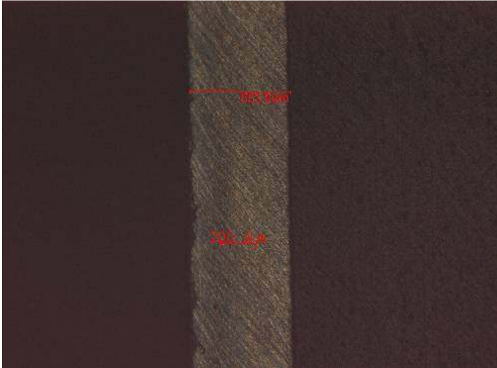
Fig.32 Coating thickness of the sample back 50X
